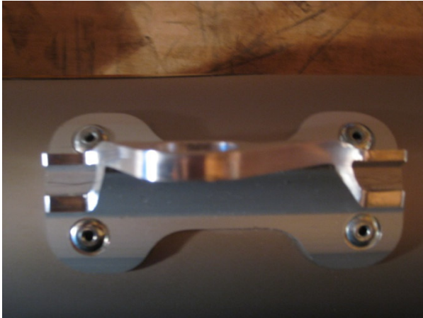
Picture of pipe mounting brackets held on only by rivets.
