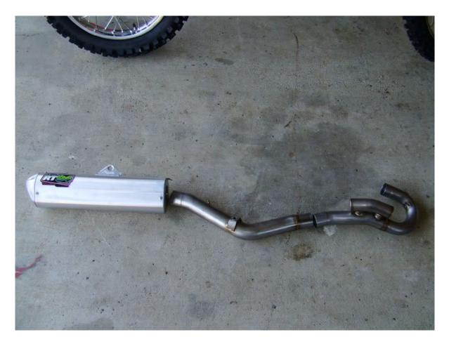
Installation was very easy. Bolt the exhaust flange collar to the head, slip the header over the collar, and install the springs. Then slide the mid-pipe on, bolt it up to the subframe, slide the muffler on the mid-pipe, and bolt it up. Make sure everything is lining up good, and tighten it all to spec. I must add that the slip-fit joints at the header/mid-pipe and mid-pipe/muffler are very tight and secure (no clamps is a bonus). I don't anticipate any leaking there.
